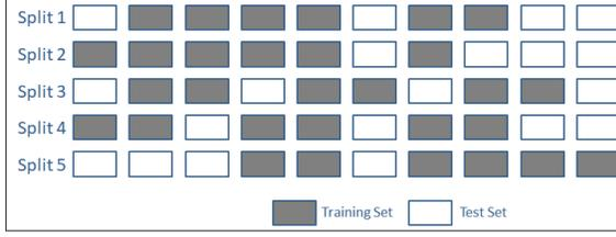
Fig. 3. Shuffle split dataset with the 60% training set and 40% test set.
